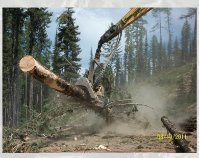
FIGURE 3: Dangle-head processor
